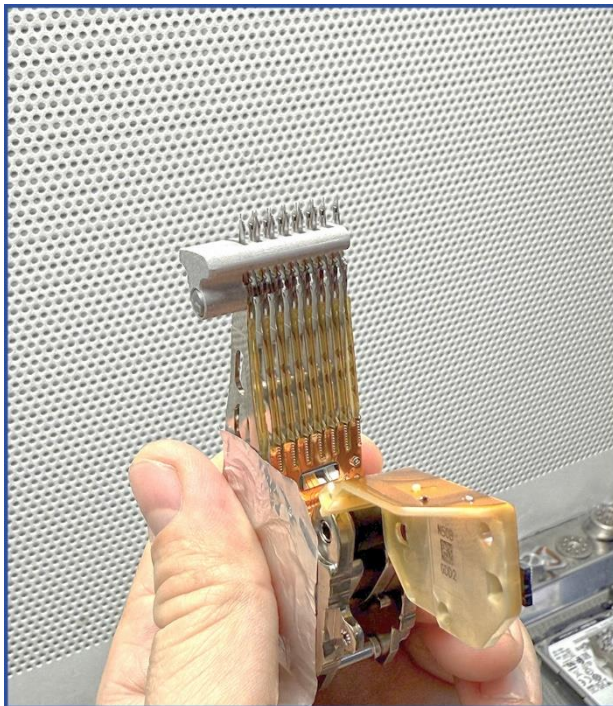
(HSA and the magnet secured with the aluminum tape)
